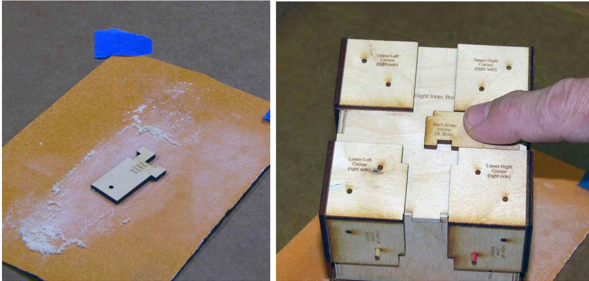
Perform the test fitting for all of the slider holders on each face of the box. Another step that you can take to prevent the slider holders from catching is to bevel the back edge of the slider holder that extends over the corner of the box.
